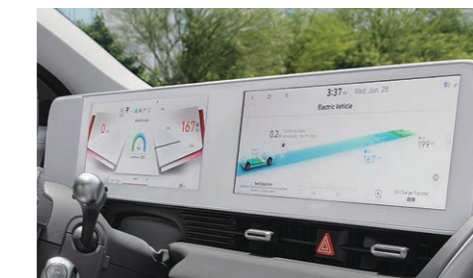
12.3" Instrument cluster & touchscreen displays
